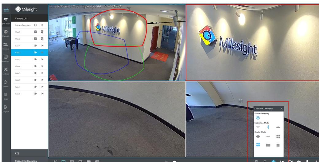
Click icon "Fisheye Client-side Dewarping" to pop up the "Client-side Dewarping" panel. You can set the Installation Mode and Display Mode according to your own needs. For instance, in 1O3R mode, the viewing angle of R1 image can be adjusted according to the corresponding color border (red). [For more information about the Dewarping Panel, see Part 4 of this article.](#)
